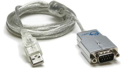
Simplifies configuration of Acromag I/O Modules ♦ Enables configuration via USB port
