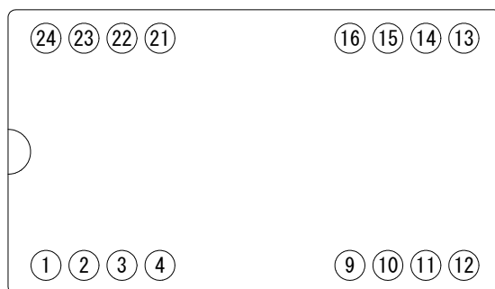
<Pin Location (Top View) >
