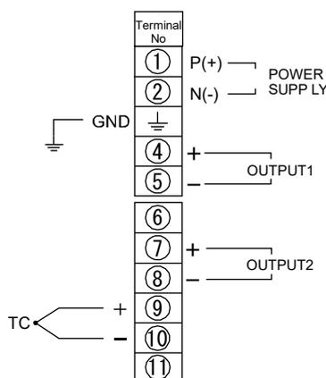
Note: For the single output model, the OUTPUT2 shown should be interpreted as N.C.
