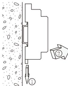
Push the slide clamp downward with a flat-head screwdriver bit or the like (①), and pull the lower part of the socket toward you (②).
