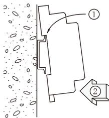
Hold the socket with the slide clamp facing down. Hook the upper edge of the cavity in the rear of the socket over the upper blade of the rail (①), then push the lower part of the socket against the lower blade of the rail so as to make the slide clamp engaged firmly with the rail (②).
