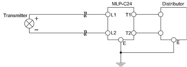
NOTE: If the distance from the MLP device to the equipment to be protected is over 10 meters, it is recommended that an additional MLP device adjacent to the equipment to be protected should be installed.
