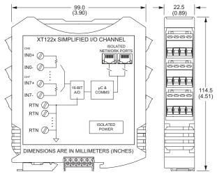
8-channel differential analog voltage input
