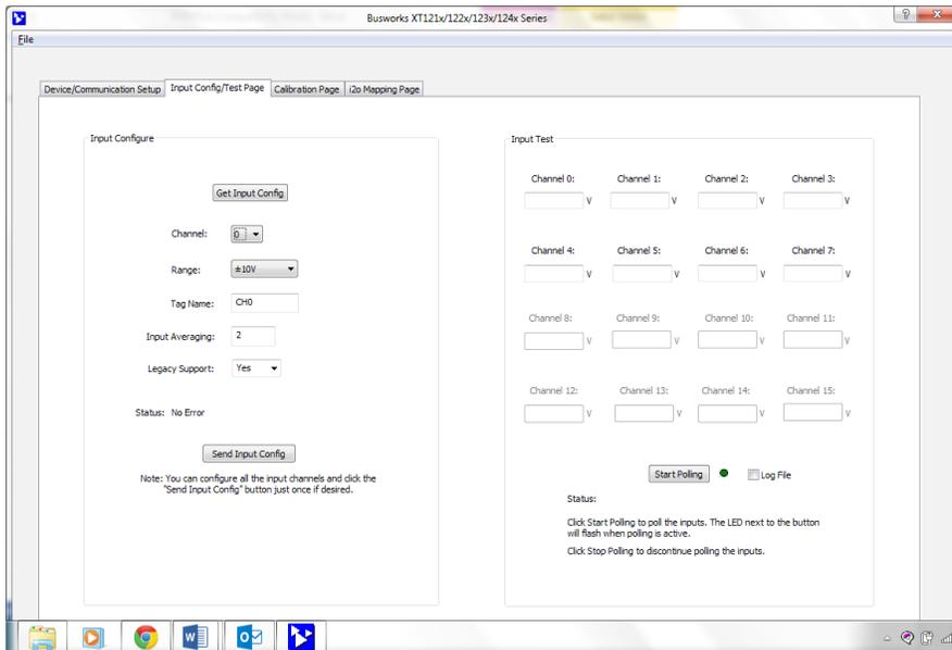
BusWorks XT software (download free from [www.acromag.com](http://www.acromag.com)) allows you to configure I/O modules offline with USB or save the configuration file and download settings into units later at your convenience.
