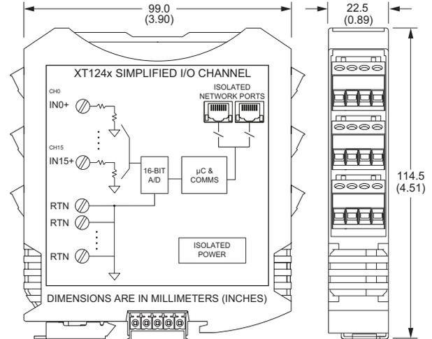
16-channel single-ended analog voltage input ♦ Modbus TCP/IP, Ethernet/IP, Profinet, or i2o communication
