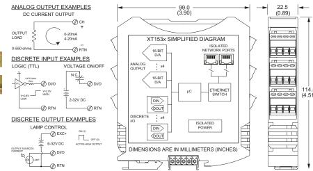
4 analog current outputs, 4 discrete I/O channels ◆ Modbus TCP/IP, Ethernet/IP, Profinet, or i2o communication
